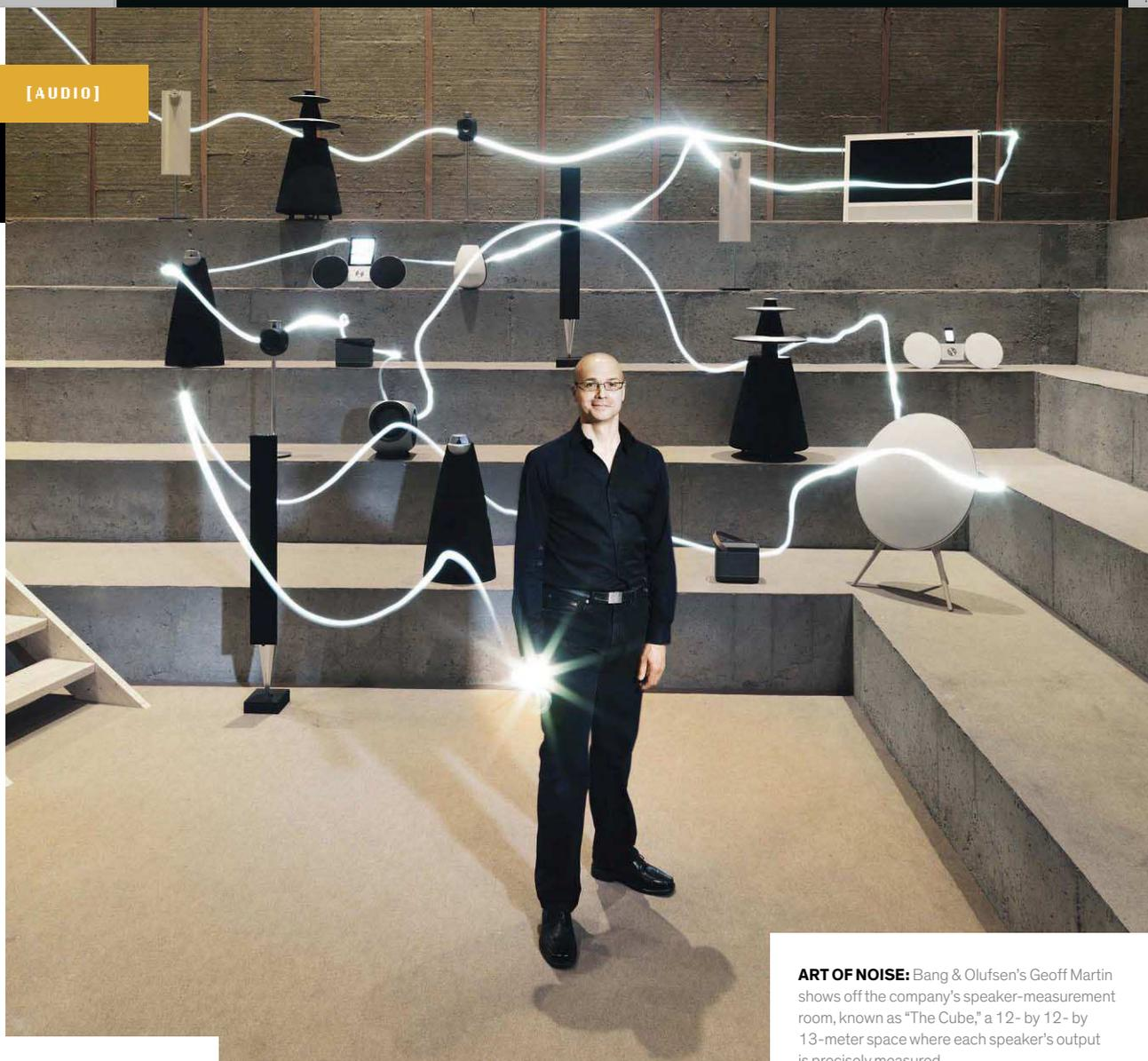
**ART OF NOISE:** Bang & Olufsen's Geoff Martin shows off the company's speaker-measurement room, known as "The Cube," a 12- by 12- by 13-meter space where each speaker's output is precisely measured.
