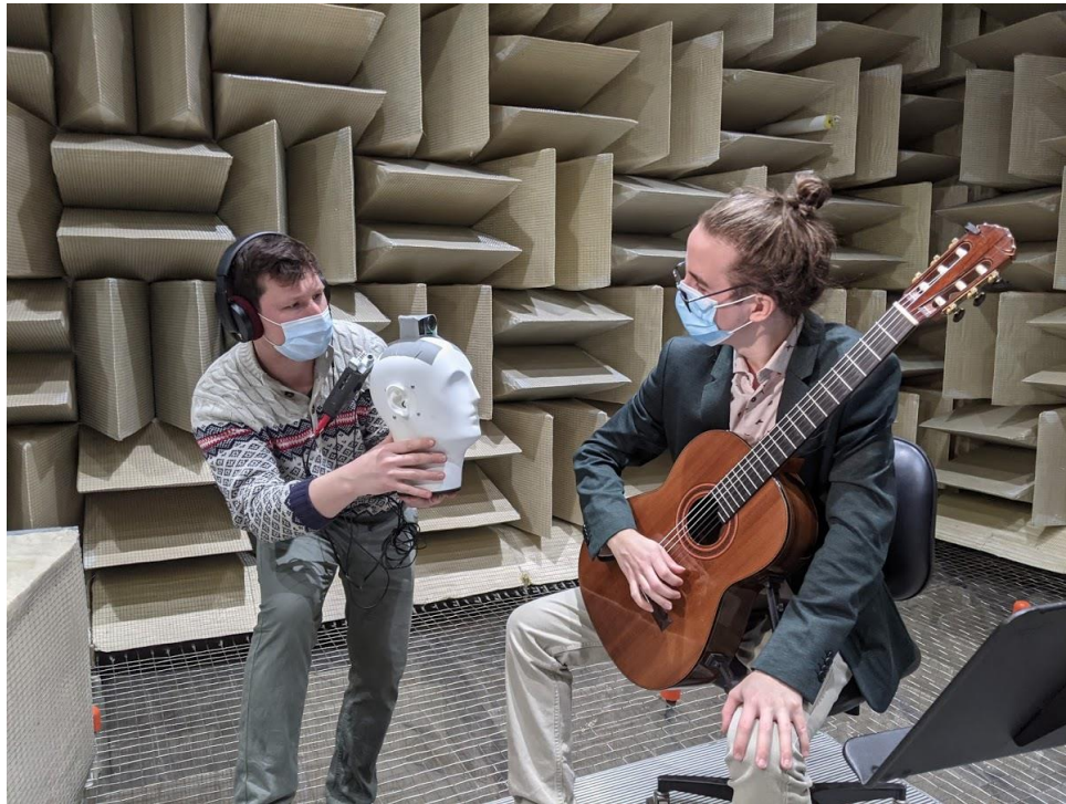
Figure 2: Pierre Grandjean holds the binaural enthusiast head while preparing a classical guitar audio/video recording in an anechoic room
